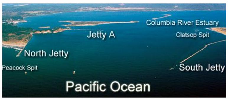
The 6.5-mile south jetty helps contain and trap the shifting sand deposits at the mouth of the river. It was instrumental in the formation of Clatsop Spit, which was a partially submerged shoal before the construction of the jetty. It is located north of the beginning of the south jetty.
